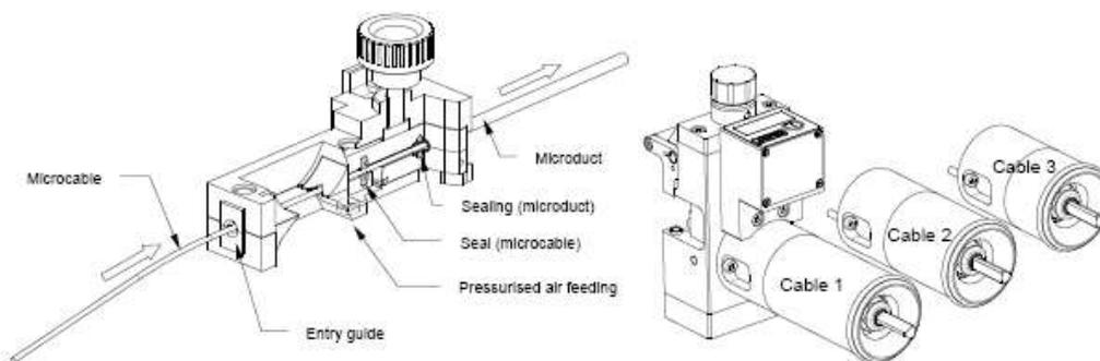
**Figure 7:** Cartridge design and modular concept
