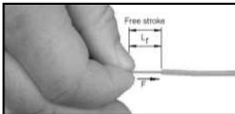
**Figure. 3:** Free stroke  $L_f$
