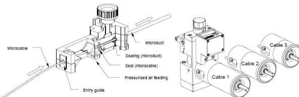
**Figure 7:** Cartridge design and modular concept
