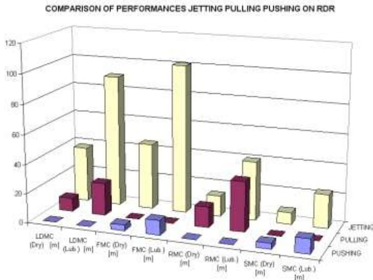
**Figure 6:** Performance comparison chart between Jetting, Pushing & Pulling
