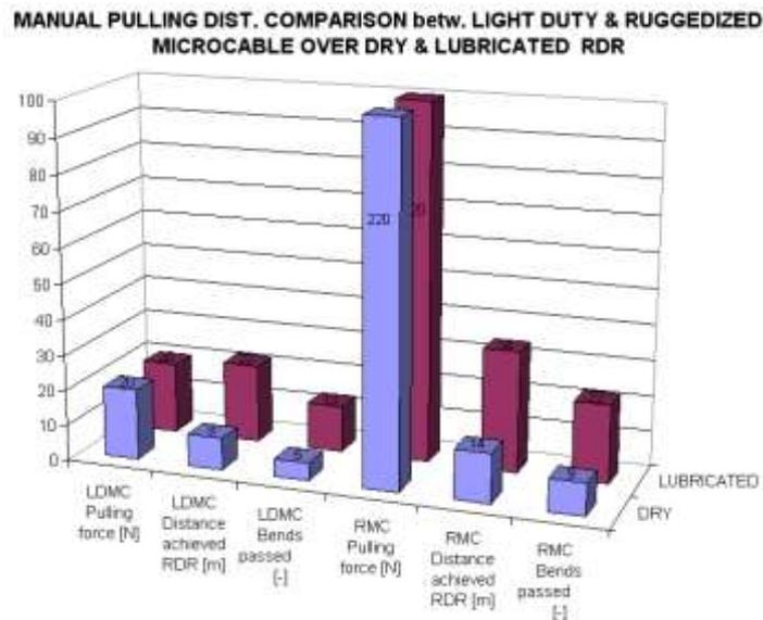
**Figure 2:** Comparison chart for manual pulling
