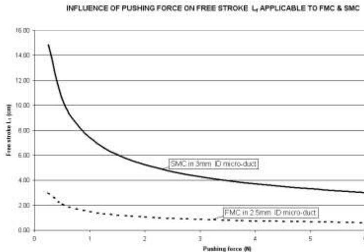
**Figure 4:** Free stroke  $L_f$  versus manual push on stiff and flexible micro-cable
